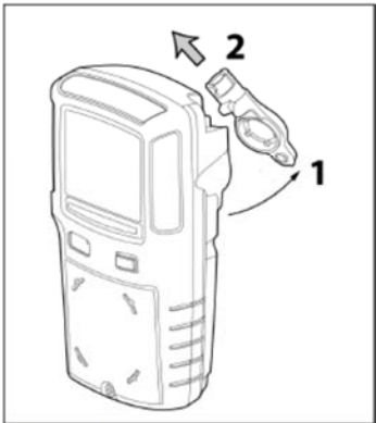
Figure 13. Removing the Pump Filters
