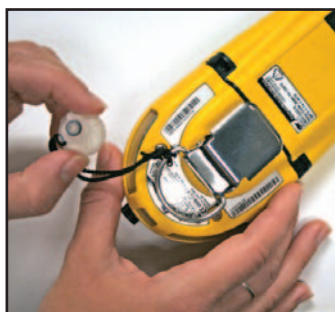
Attaching the Auxiliary Filter to the GasAlertMicro 5
