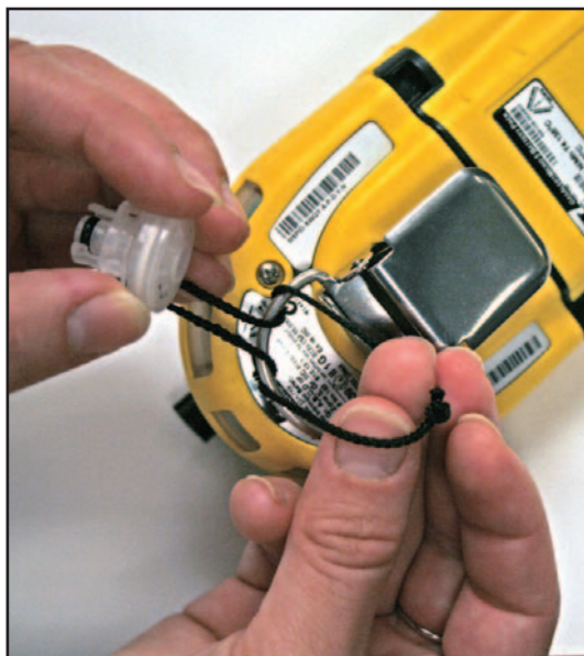
Attaching the Auxiliary Filter to the GasAlertMicro 5
