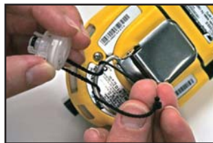
Attaching the Auxiliary Filter to the GasAlertMicro 5
