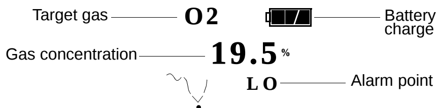
Figure 4: LCD in Alarm Adjustment Mode
